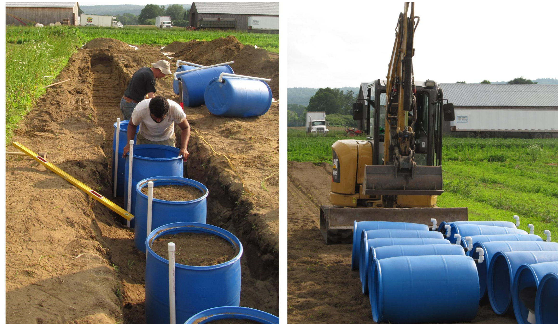
Figure 4. Tank lysimeters intercept and store all soil leachate passing through the enclosed soil column. Leachate is periodically collected for contaminant analysis.
